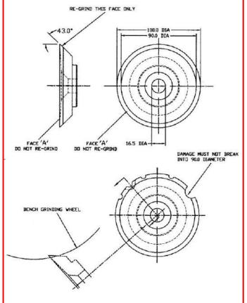
Examine set of chipper disc blades for damage. If front face 'A' is worn, blade must be scrapped. If chips have broken off cutting edge they can be redressed provided that they do not go inside 90mm diameter area.
