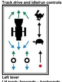
Left lever LH track: forwards – backwards Right lever RH track: forwards – backwards Lever with red knob Engine idle/run: slow - fast
