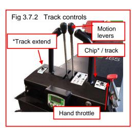
Note: Drive with track motors at rear when possible.
