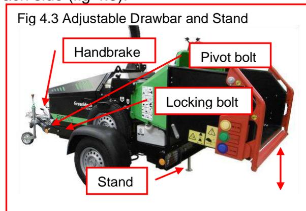
**⚠ CAUTION!** Infeed chute must not be used at less than 600mm from ground (fig 3.4.3). Adjust drawbar of Road tow models as necessary.
