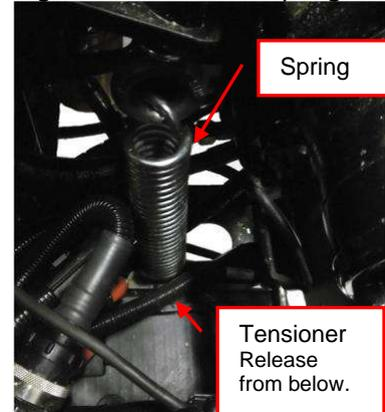
Fig 5.4.2 Feed roller lift
