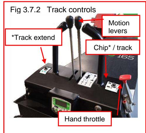
**Note:** Drive with track motors at rear when possible.
