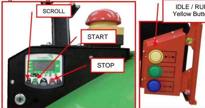
Fig 5.2.2 Engine Controls
