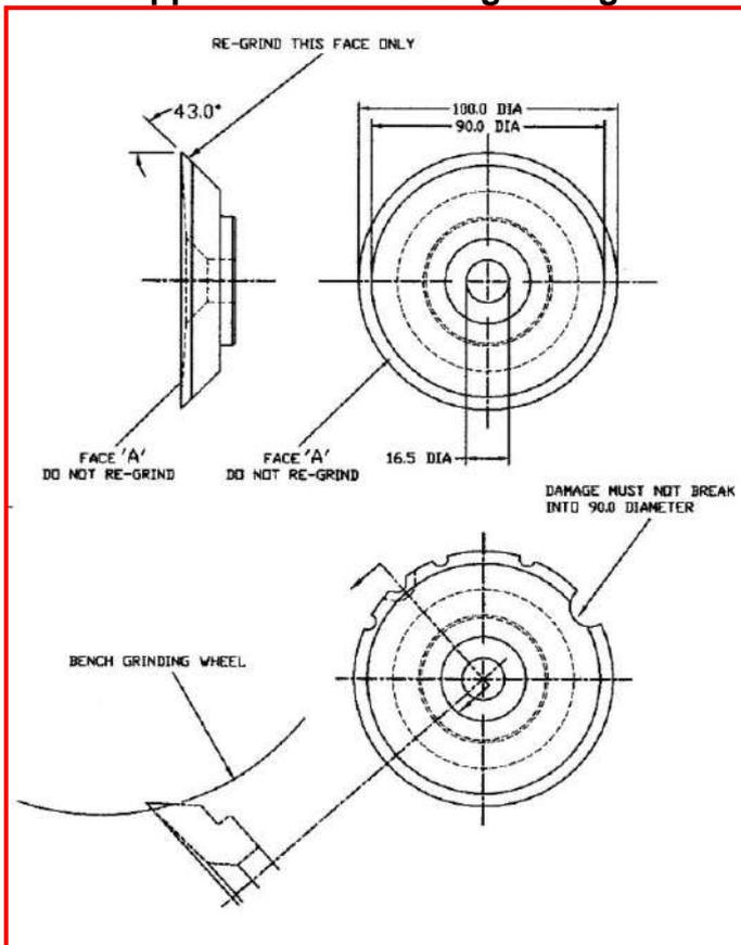
Examine set of chipper disc blades for damage. If front face 'A' is worn, blade must be scrapped. If chips have broken off cutting edge they can be re-dressed provided that they do not go inside 90mm diameter area.
